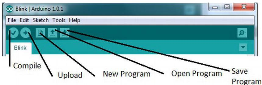
*Figure 1-14. Toolbar with function breakout.*
