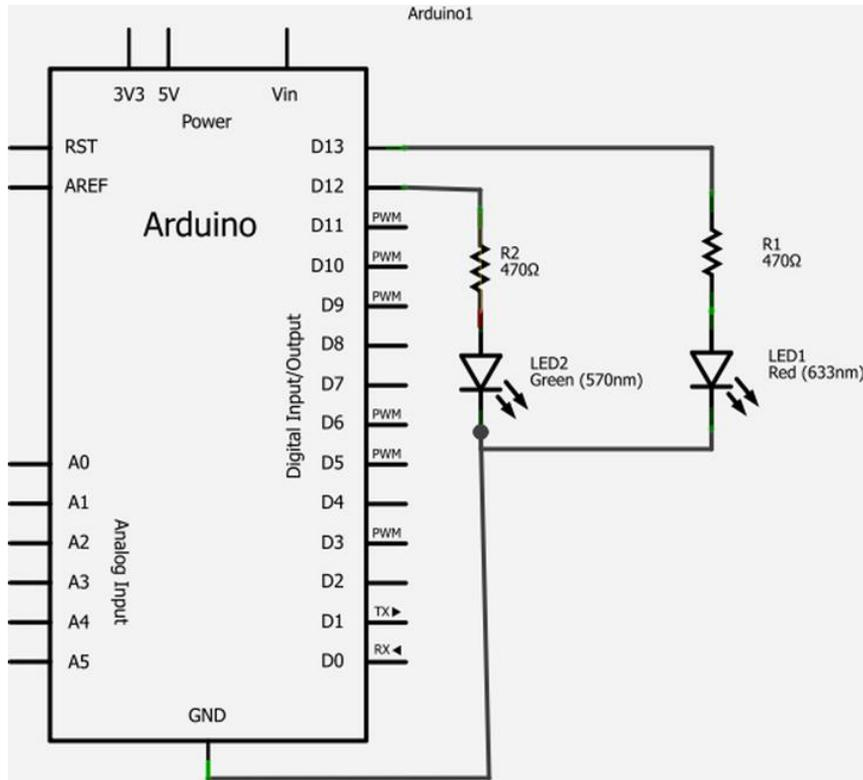
Figure 4-4. The Schematic for the Alternate Blink program.
