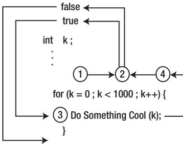
Figure 5-1. The Program Flow Using a for Loop.
