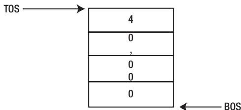
**Figure 6-4.** *The Program Stack With a Memory Address on the Stack.*
