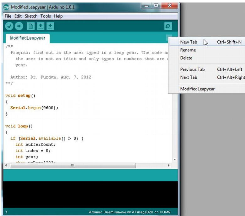
Figure 7-5. Adding a second source file to a sketch.
