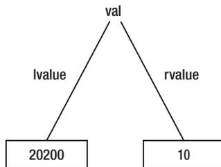
*Figure 3-4. The lvalue-rvalue diagram after processing the assignment statement.*
