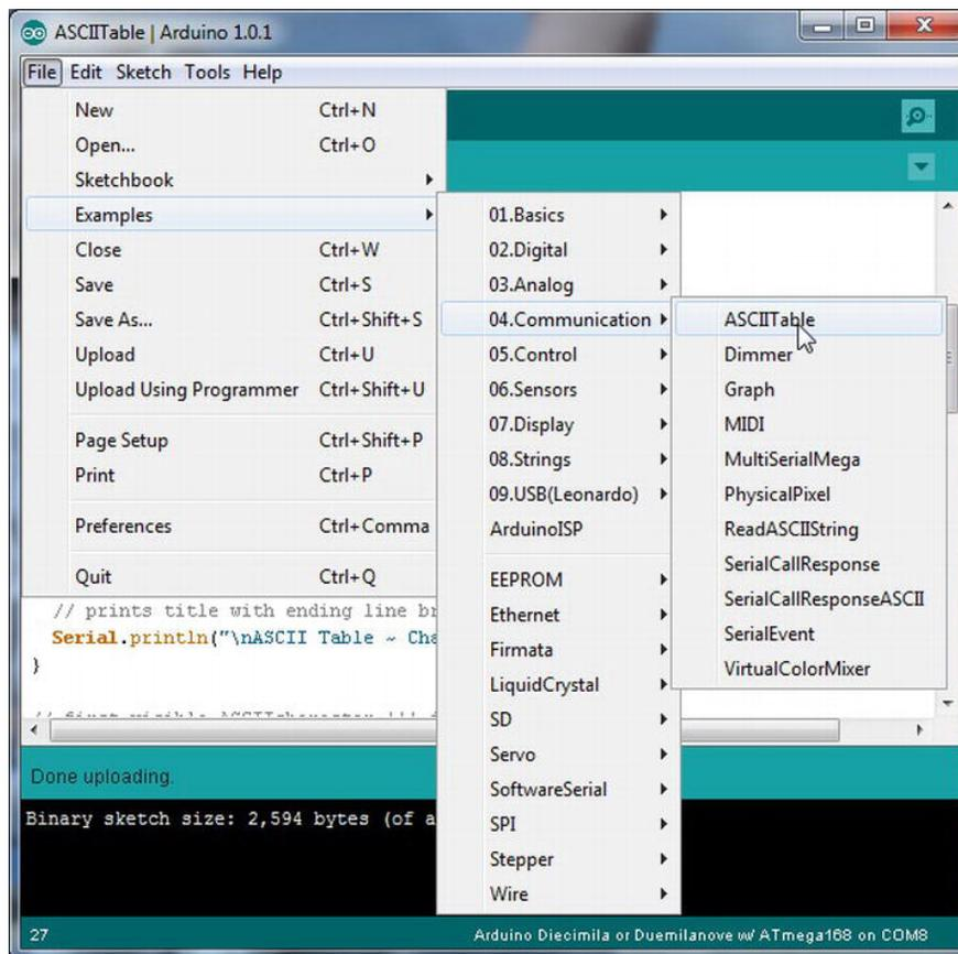
Figure 3-1. Loading the ASCII Table sample program.
