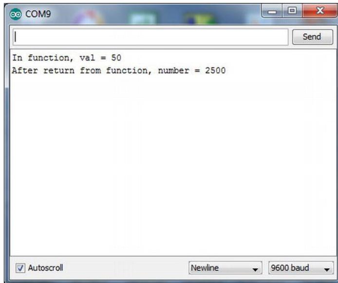
*Figure 9-5. Sample run of pointer to function program.*
