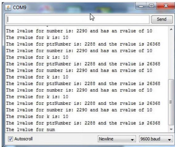
*Figure 8-7. Using the indirection operator in an assignment statement.*
