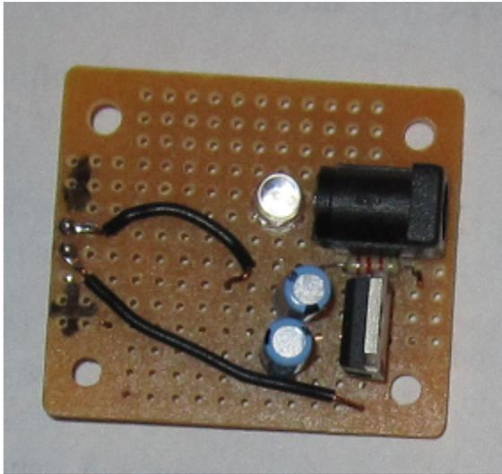
*Figure B-1. A small voltage regulator circuit.*
