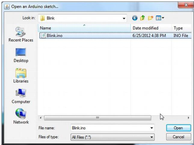
*Figure 1-12. Loading the Blink.ino source code file.*
