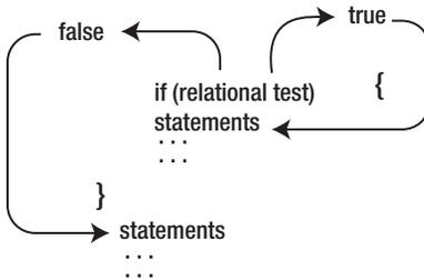
Figure 4-1. Execution Paths for `if` Test.
