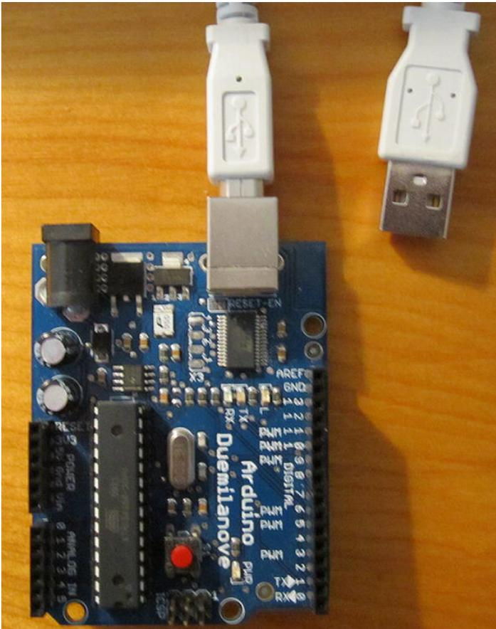
Figure 1-6. The  $\mu$  board with USB cable attached.
